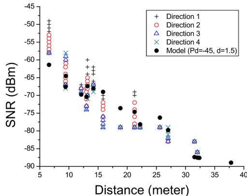
Figure 6: Measurements vs. the RSS model of WirelessHART device.
