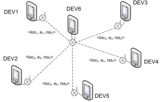
**Figure 2: Illustrating collaborative estimation with 5 HartFi devices**
