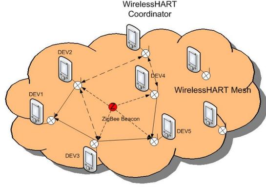
Figure 3: Leveraging ZigBee devices in localization
