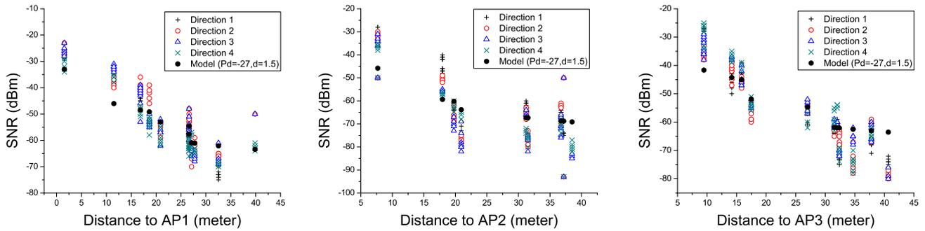
Figure 5: Measurements vs. the RSS model of three Wi-Fi APs.
