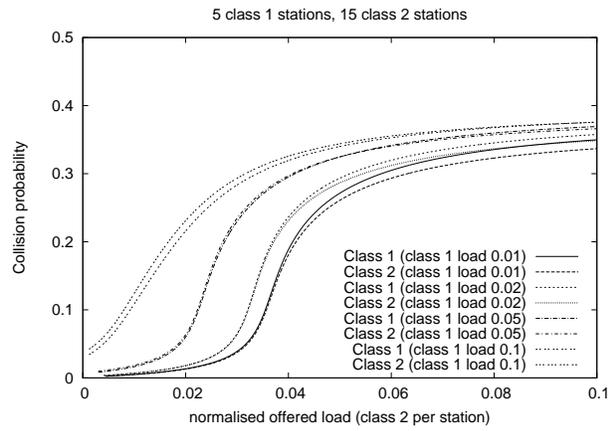
Fig. 15. Overall throughput and per station collision probabilities for two classes of stations with class 1 offering fixed per station load,  $n_1 = 5$ ,  $n_2 = 15$ .
