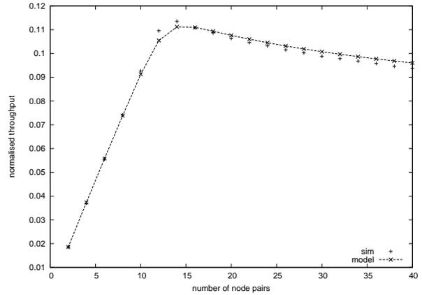
Fig. 7. Throughput for station-pairs sending 64kbps on-off traffic streams.
