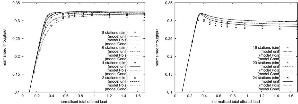
Fig. 3. Throughput as the traffic arrival rate is varied. At rates below those shown there is agreement between the model and simulation. Results for the three load relationships (uniform, Poisson and conditional) presented in Section III-D are shown.
