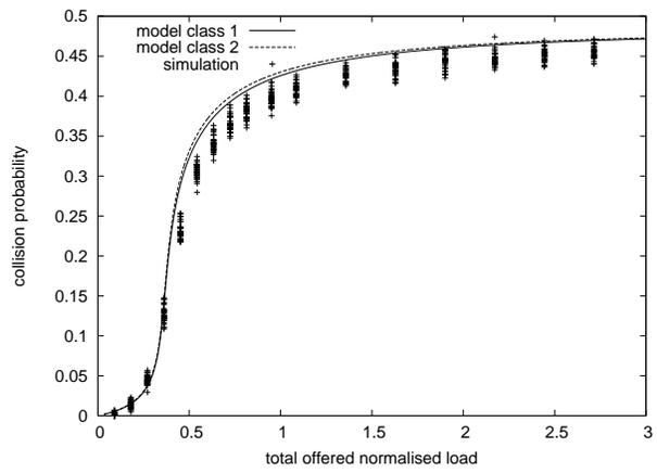
Fig. 6. Normalized per-station throughput and collision probability, where  $n_1 = 12$ ,  $n_2 = 24$  and the offered load of a class 2 station is  $1/4$  of a class 1 station.
