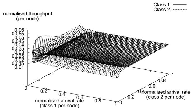
Fig. 13. Per-station throughput for two classes of stations offering different loads,  $n_1 = 5$ ,  $n_2 = 15$ .
