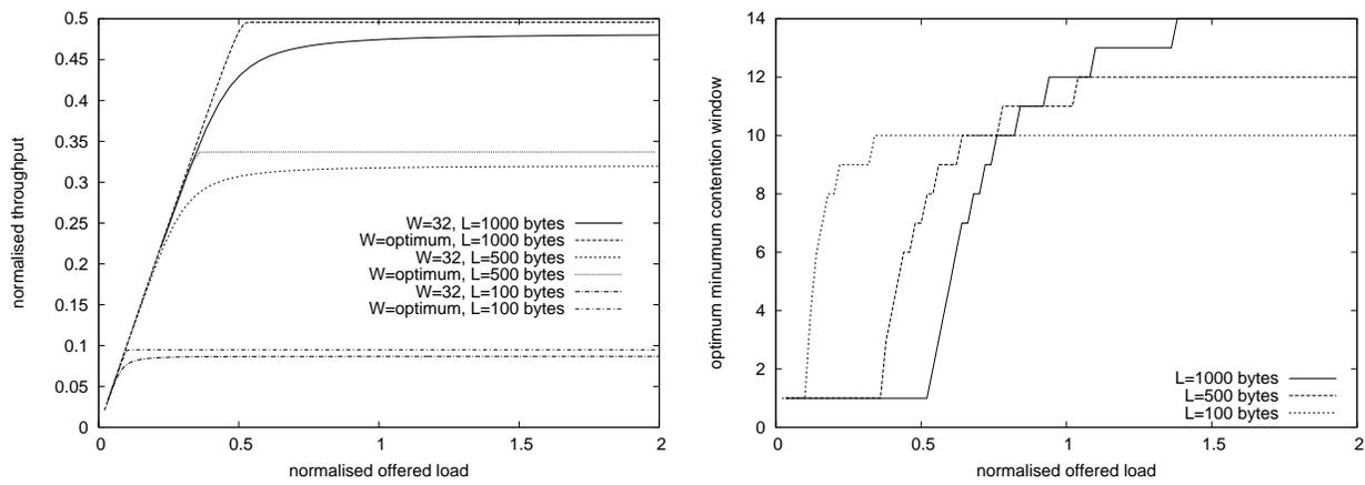
Fig. 8. Throughput for 2 stations as the offered load is varied for  $CW_{min}=32$  and with  $CW_{min}$  optimized. Results for various payload sizes,  $L$ , are also shown.
