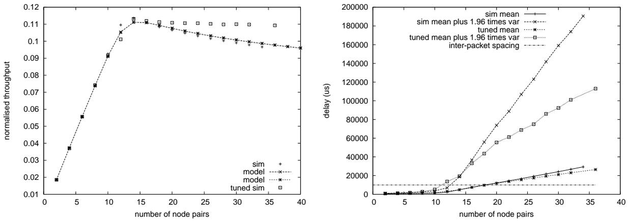
Fig. 12. Throughput and average MAC delays for station-pairs sending 64kbps on-off traffic streams.
