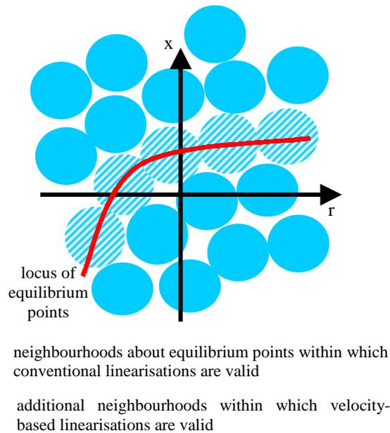
Figure 1 - Validity of conventional and velocity-based linearisations
