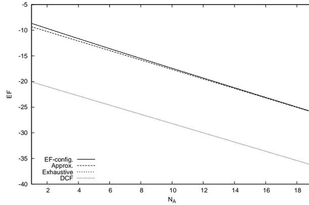
Figure 5.3: EF performance for a heterogeneous WLAN with two types of interfaces: A+B
