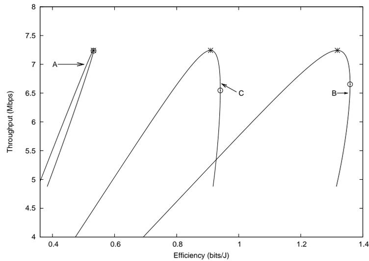
Figure 5.2: Trade-off imposed by the energy features of the WLAN interfaces
