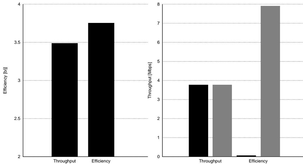
Figure 2.1: Throughput and Energy-Efficiency performance of a WLAN with two stations modeled after interfaces A (grey) and B (black) from Table 2.1.
