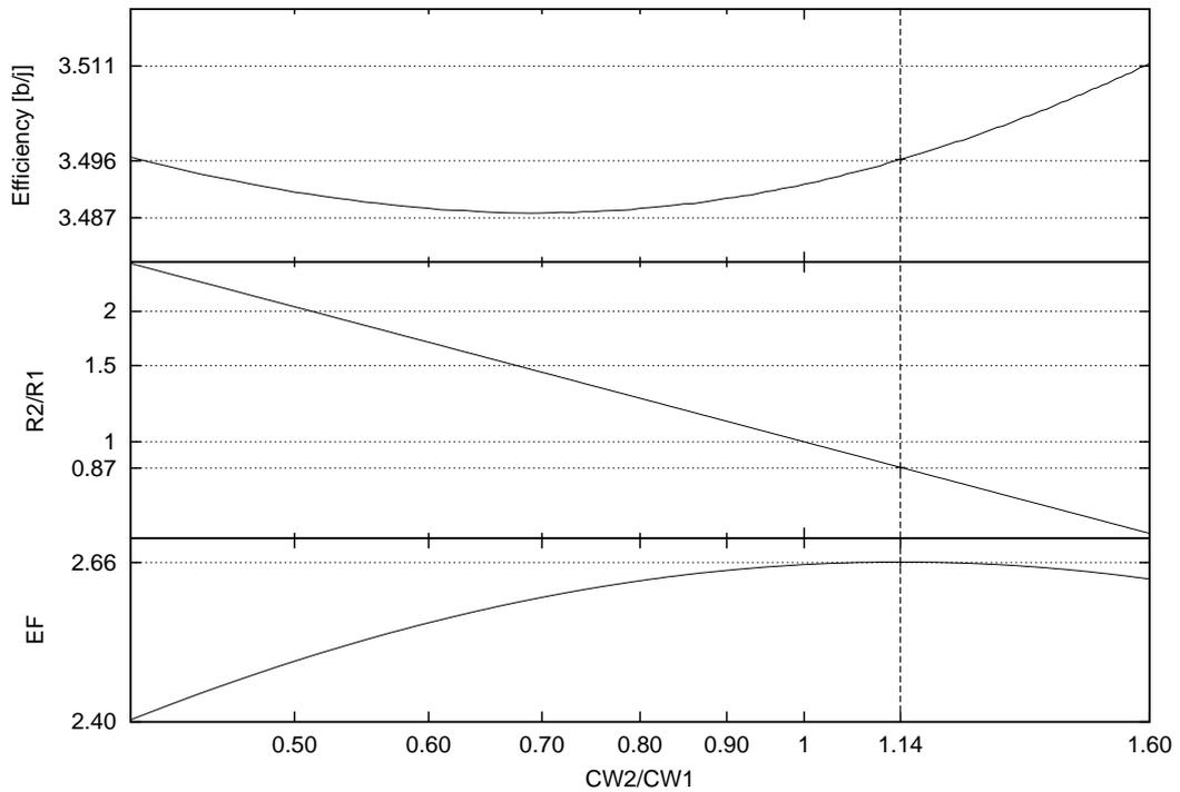
Figure 2.2: Total efficiency, throughput ratio and EF performance of a WLAN with two stations for different  $CW$  configurations.
