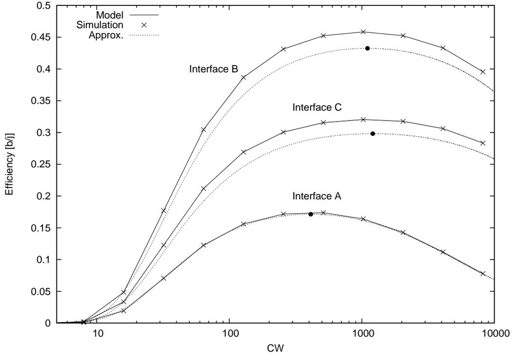
Figure 3.2: Per-station efficiency  $\eta_i$  for a WLAN with  $N = 30$  stations.
