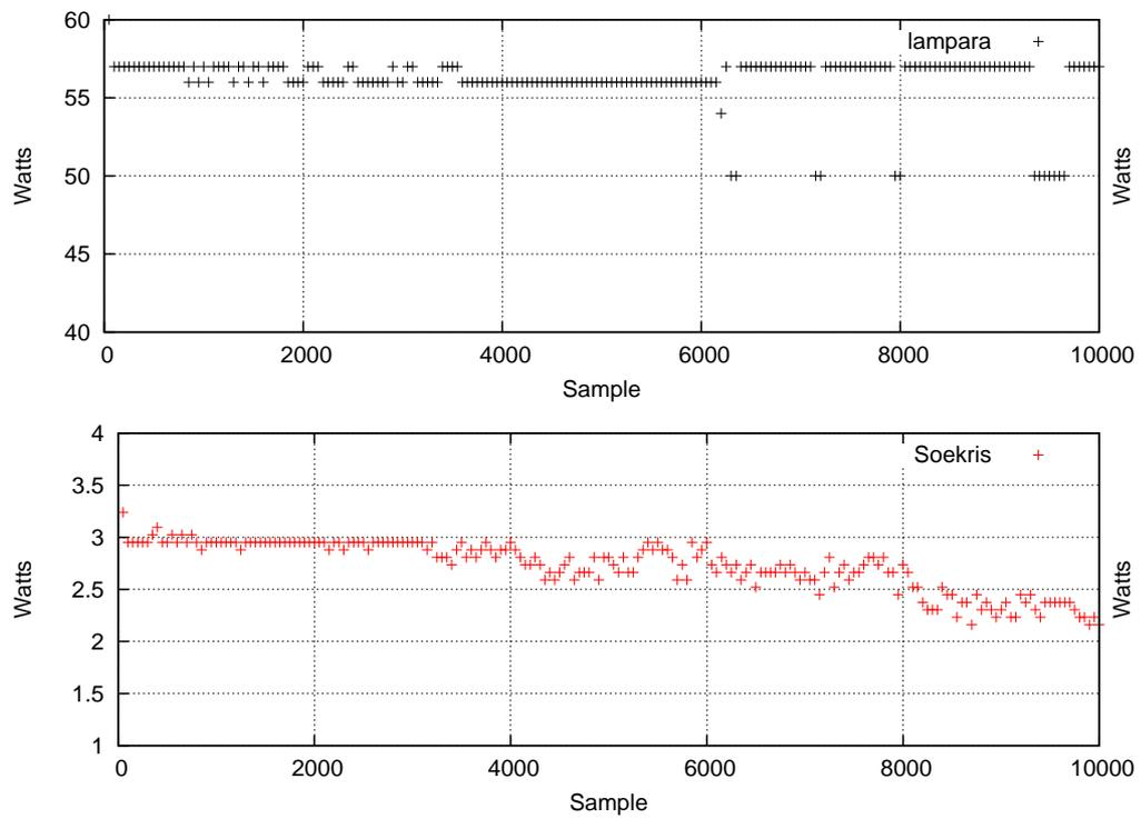
Figure 6.3: Measurements on a Soekris box for different device's uptime
