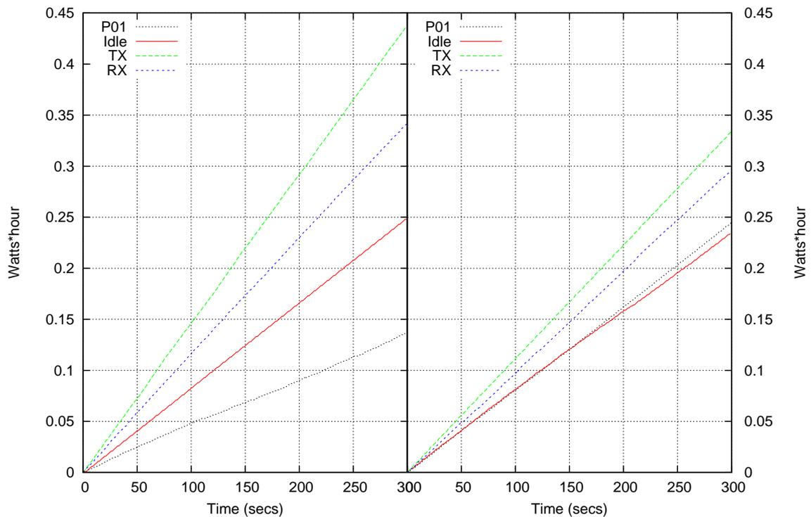
Figure 6.2: Measurements on a Soekris box for different device's uptime
