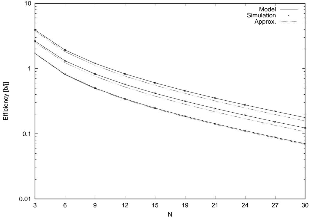
Figure 3.1: Overall energy efficiency  $\eta$  of a heterogeneous WLAN with  $N$  stations.
