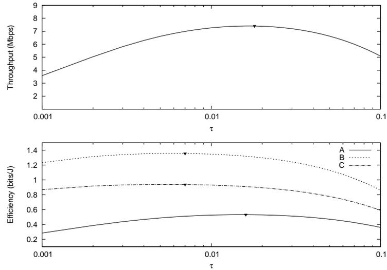
Figure 5.1: Energy efficiency and throughput vs.  $\tau$ .
