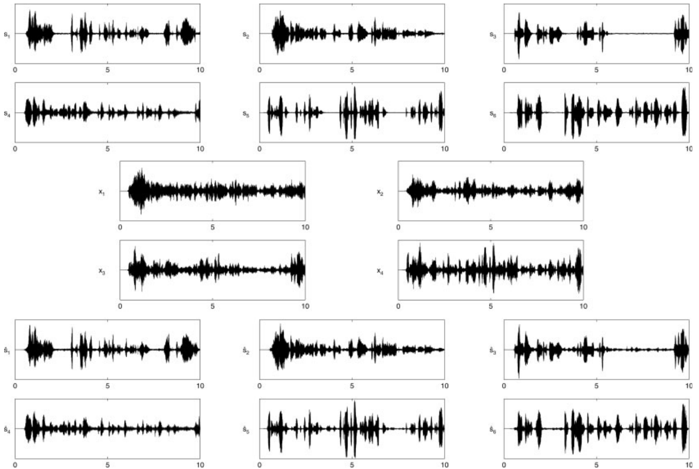
Figure 4. Separation of 6 sources from 4 mixtures using the Soft-LOST algorithm (O’Grady and Pearlmutter, 2004b). The plots above show 10-s clips of six acoustic sources s_1, \dots, s_6 , 4 mixtures x_1, \dots, x_4 and 6 source estimates \hat{s}_1, \dots, \hat{s}_6 , where sound wave pressure is plotted against time in units of seconds. The signal-to-noise ratios of the estimated sources in dB are as follows: 10.5845, 13.3895, 13.7402, 8.9102, 15.2732 and 11.3213.
