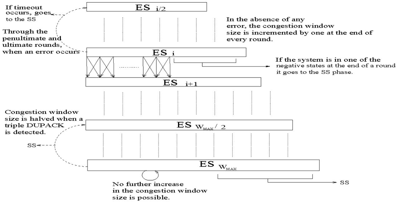
Fig. 3. The transition between the Errorless rounds through the Penultimate and Ultimate rounds for a range of congestion window sizes. The transition between  $ES_i$  and  $ES_{i+1}$  takes place only at the end of the round.
