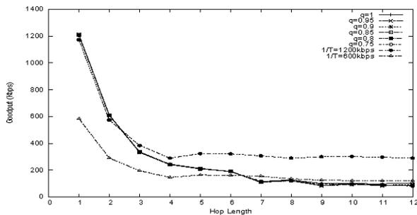
Fig. 7. Goodput vs Hop Length (for fixed  $p=0.01$ ) with two state Markov error model.
