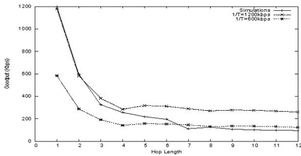
Fig. 5. Goodput vs Hop Length (for fixed  $p=0.01$ ) with uniform error model.
