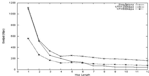
Fig. 6. Goodput vs Hop Length (for fixed  $p=0.05$ ) with uniform error model.
