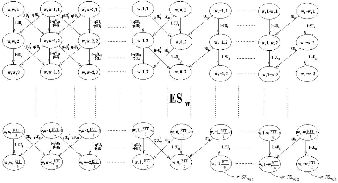
Fig. 2. An Errorless round ( $ES_w$ ) with congestion window size  $w$ . We denote  $(1 - p_e)U_t$  by  $U_t$  for simplicity of exposition. Here,  $SS_{w/2}$  denotes the slow start phase with  $SSThresh$  equal to  $\frac{w}{2}$ .
