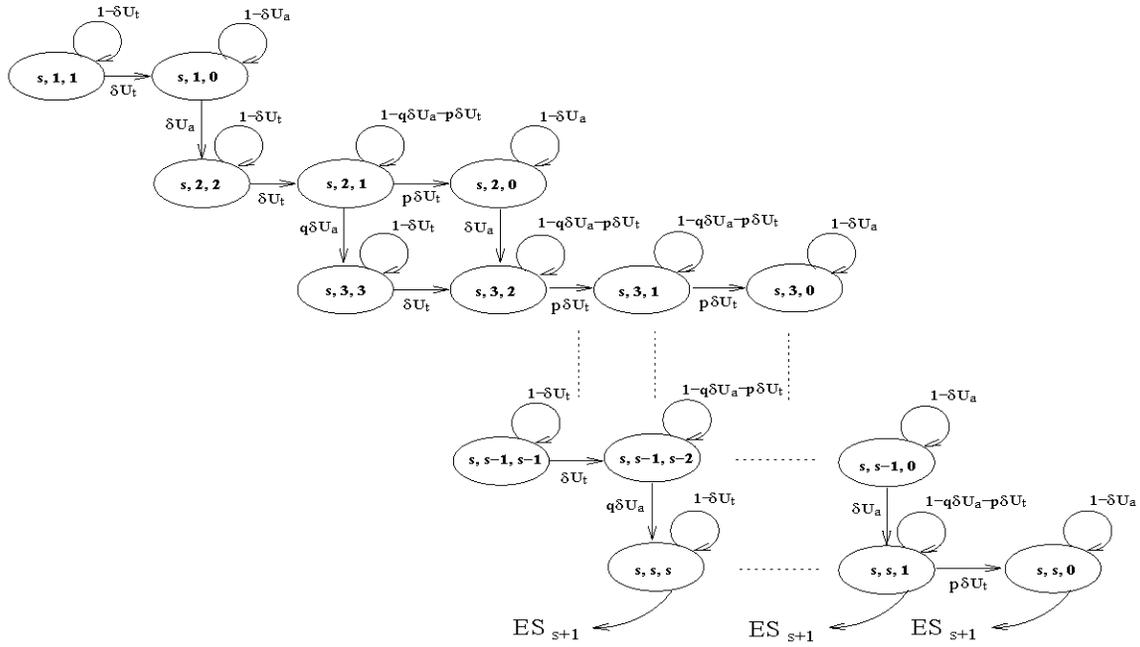
Fig. 1. Slow start phase ( $SS_s$ ) with the value of  $SSThresh$  being  $s$ , for various possible values of  $w$  and  $l$ . Here,  $ES_{s+1}$  denotes the Errorless round with congestion window size  $s + 1$ .
