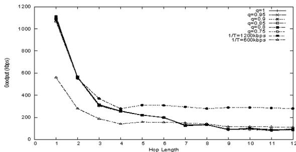
Fig. 8. Goodput vs Hop Length (for fixed  $p=0.05$ ) with two state Markov error model.
