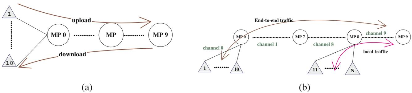
**Fig. 2** Illustrative wireless multi-hop scenarios. **a** Scenario 1: end-to-end traffic only. **b** Scenario 2: with local traffic
