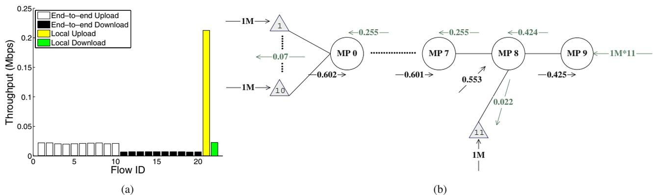
**Fig. 4** CBR results without TXOP for scenario in Fig. 2b with one client station at  $MP_8$ . Per flow throughput is shown in Fig. 4a. Per hop aggregate throughput (in Mbps) is plotted in Fig. 4b. Simulation parameters listed in Table 1. Note that 0.553 Mbps
