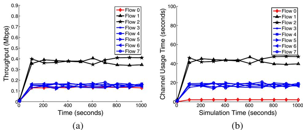
**Fig. 16** Throughput-fairness allocation when multiple PHY rates are available for the scenario in Fig. 7. The link rates between  $MP_0$  and  $MP_2$ , and  $MP_4$  and  $MP_5$  are 11 Mbps, while other link rates are still 1 Mbps. Other simulation parameters listed in
