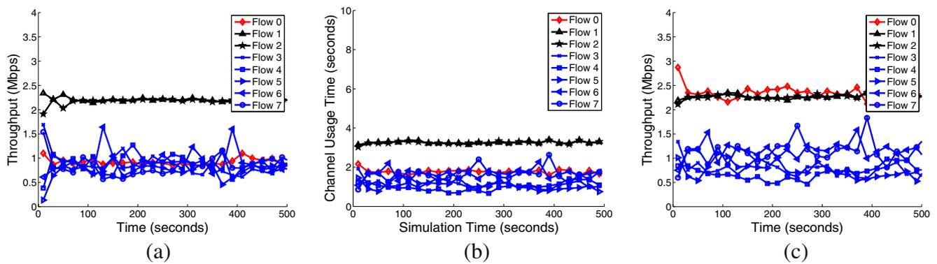
**Fig. 20** Test-bed results when the PHY rate between  $MP_0$  and  $MP_2$  and that between  $MP_4$  and  $MP_5$  are increased to be 12 Mbps for the topology in Fig. 7. While PHY rates on all other links are still 6 Mbps. Other parameters used is listed in Table 3. Note that in Fig. 20a, the throughput of flow 0 overlaps with that
