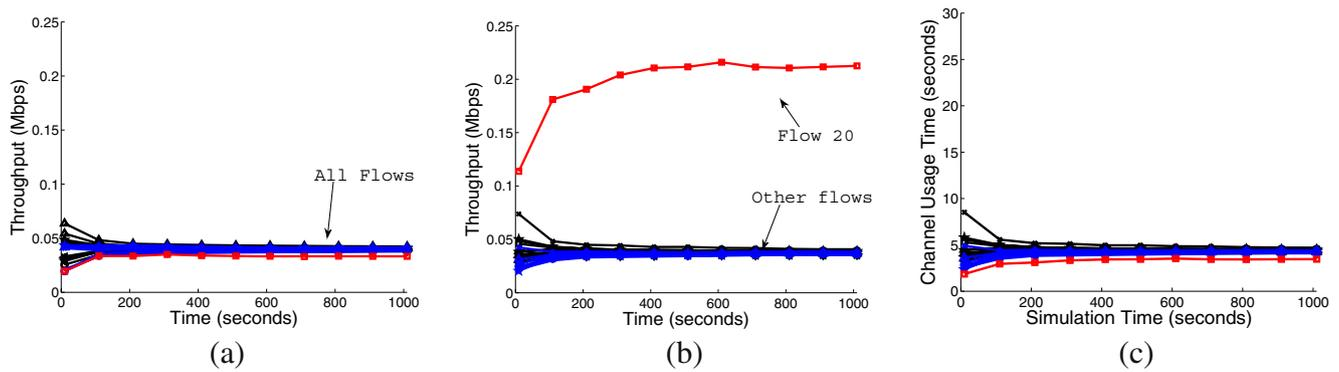
**Fig. 18** Time-based fairness allocation when multiple PHY rates are available for the scenario in Fig. 14. All the link rates from station 11 to the gateway GW are 11 Mbps, while other link rates are still 1 Mbps. Other simulation parameters listed in Table 1. Note that in Fig. 18c, we also plot the channel usage time of each
