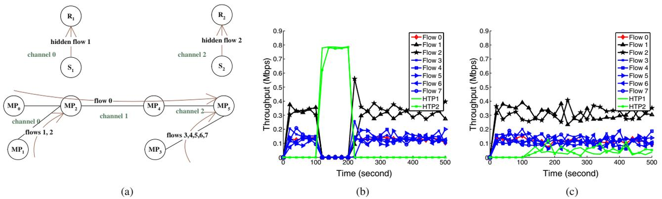
**Fig. 12** The impact of hidden terminal traffic on TCP traffic in the topology shown in Fig. 7. Simulation parameters listed in Table 1. Note that in Fig. 12b and c, the throughput of flows 3–7 overlaps. **a** Topology. **b** FTP traffic. **c** Web traffic
