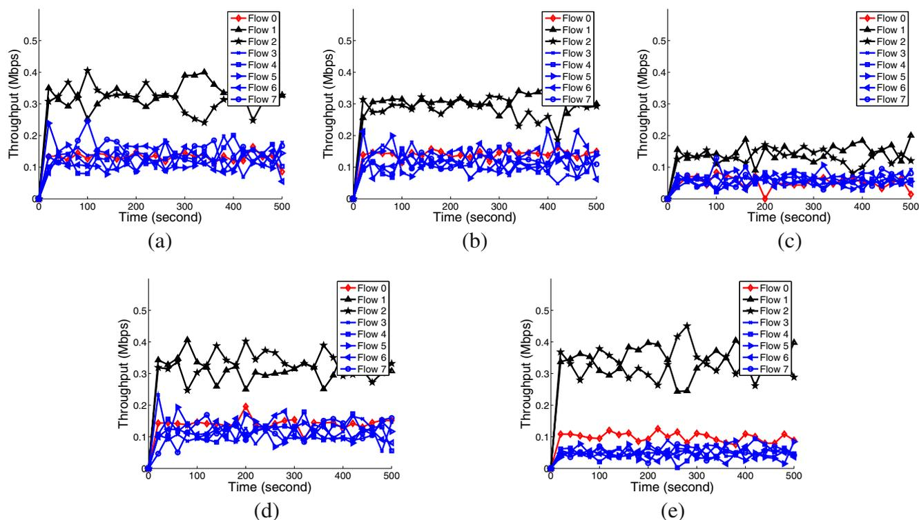
**Fig. 11** The impact of interference on TCP traffic in the topology shown in Fig. 7. Simulation parameters listed in Table 1. Note that in Fig. 11a, b, c and d, the throughput of flows 3–7 overlaps. a
