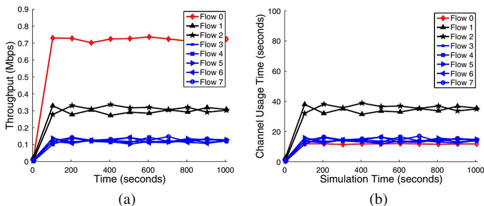
**Fig. 17** Time-based fairness allocation when multiple PHY rates are available for the scenario in Fig. 7. The link rates between  $MP_0$  and  $MP_2$ , and  $MP_4$  and  $MP_5$  are 11 Mbps, while other link rates are still 1 Mbps. Other simulation parameters listed
