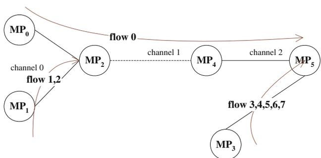
**Fig. 7** Scenario 3: a linear topology for TCP flows
