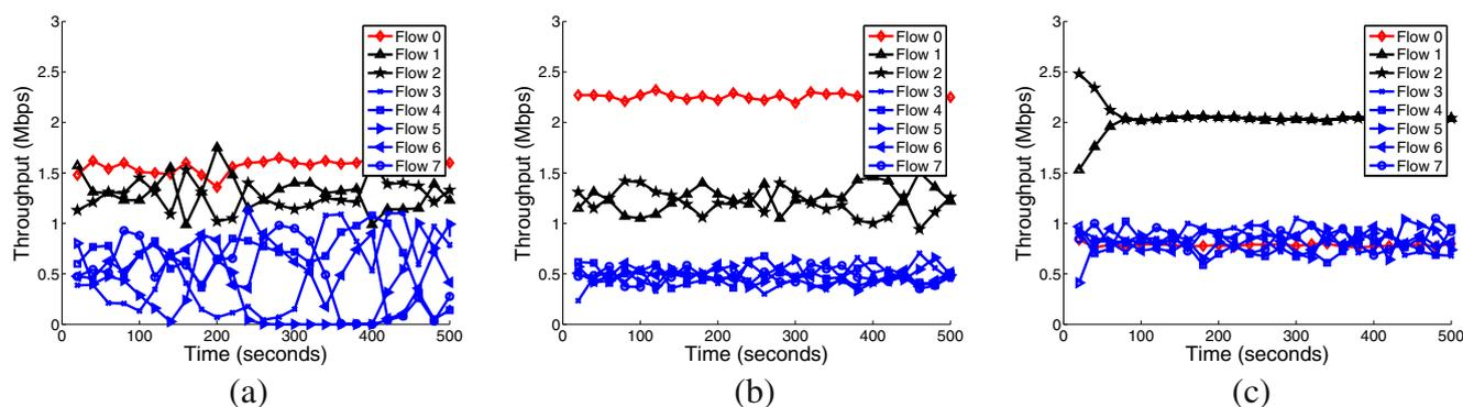
**Fig. 19** Throughput fairness: test-bed results for the topology in Fig. 7. Parameters used is listed in Table 3. Note that in Fig. 19c, the throughput of flow 0 overlaps with that of flows 3–7. **a** 802.11. **b** TCP ACK prioritisation. **c** Throughput fairness
