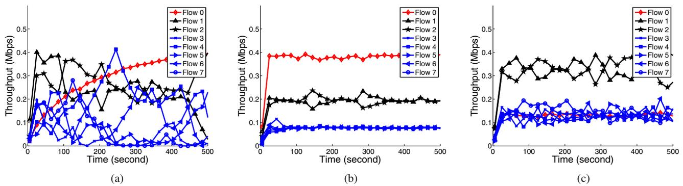
**Fig. 8** Throughput fairness: TCP results in the topology shown in Fig. 7. For prioritising TCP ACKs, TCP ACK packets are put into high priority queue with  $CW_{min} = 3$ ,  $CW_{max} = 7$  and  $AIFS = 1$ , whereas TCP data packets are put into low priority with  $CW_{min} =$
