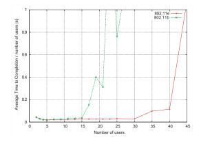
Fig. 3. Example of client-server performance in 802.11b and prioritised 802.11e WLANs.
