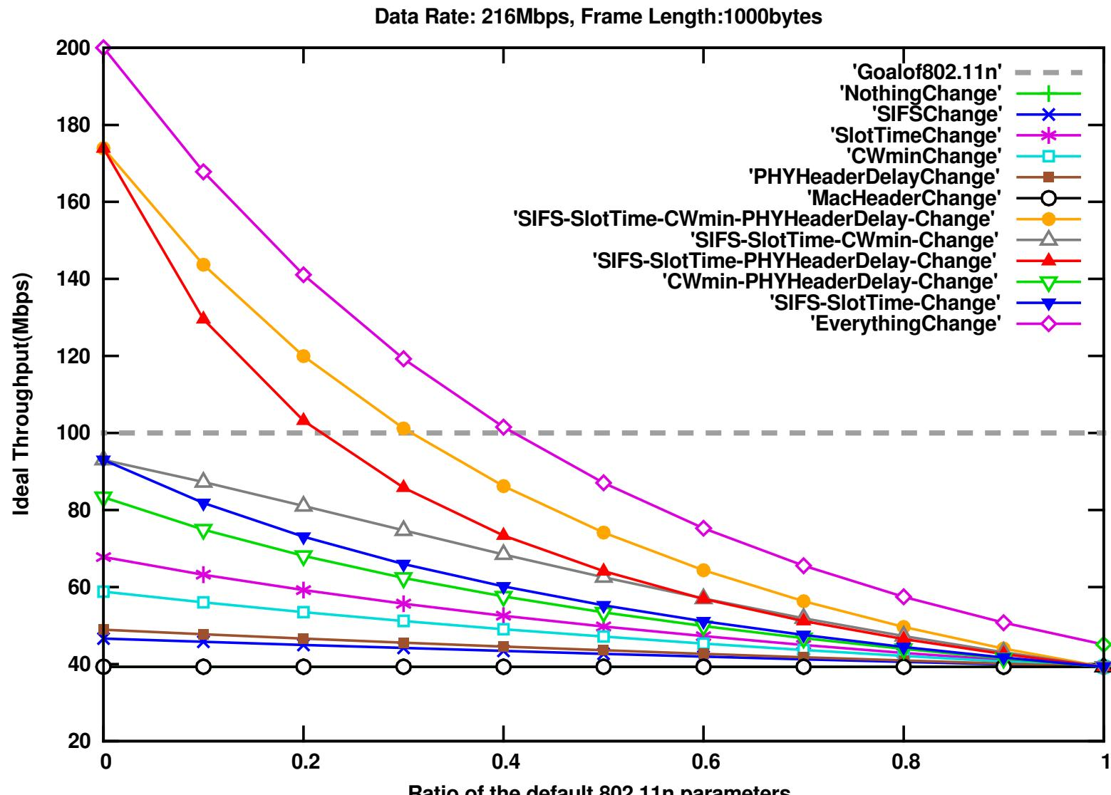
Maximum throughput while multiple parameters are modified
