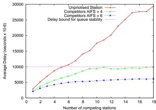
Fig. 7. Mean delay for a voice call competing with saturated stations.
