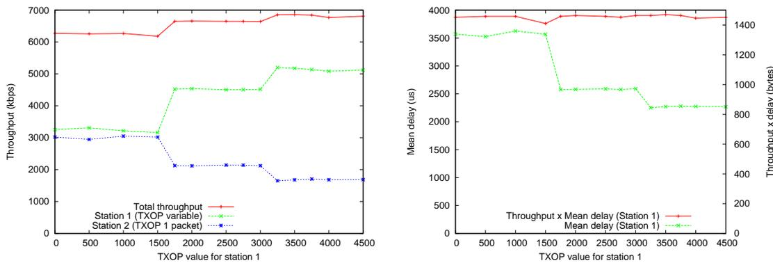
Fig. 3. The impact of TXOP on two competing saturated stations.
