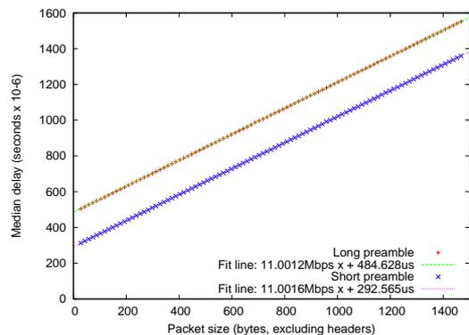
Fig. 2. Transmission time against IP packet size on a quiet network.
