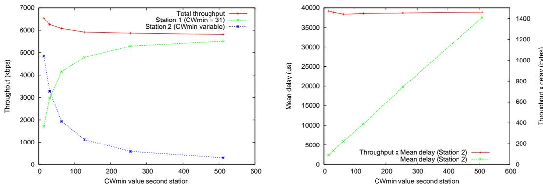
Fig. 4. The impact of CWmin on two competing saturated stations.
