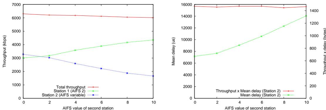
Fig. 5. The impact of AIFS on two competing saturated stations.
