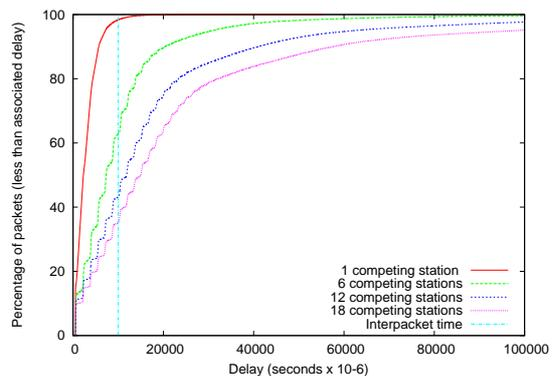
Fig. 8. CDF for the delay of an unprioritised voice call.
