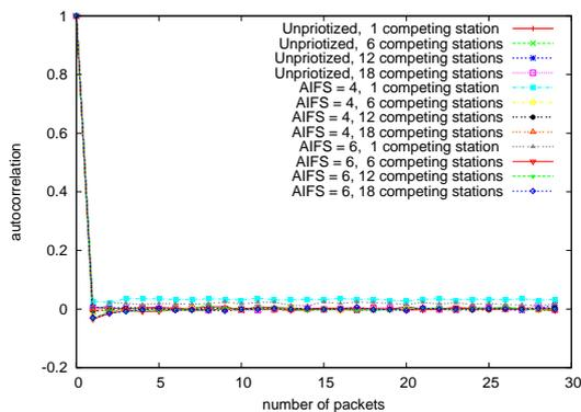
Fig. 11. Autocorrelation for sequence of packet delays.
