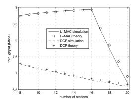
Fig. 7. Network throughput vs number of stations, comparison between the theoretical model and the simulation results.  $\beta=0.95$ . Ns-2 simulations and theory based estimates
